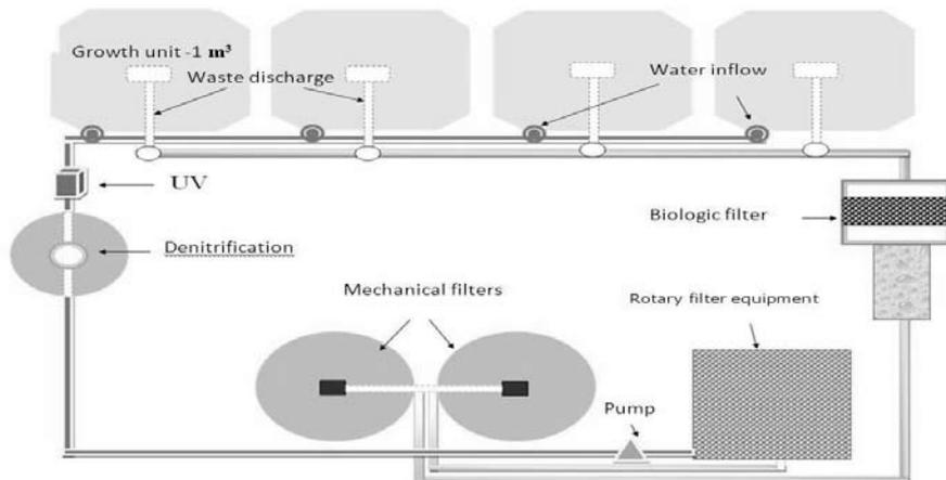
**Fig. 1.** Configuration of the experimental recirculating system
