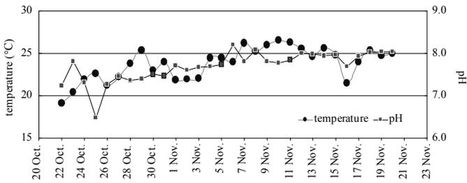
**Fig. 2.** Water temperature and pH variation during the experiment of common carp rearing in RAS
