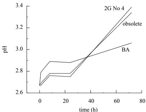
**Fig. 1.** pH versus time for Neoseptal with different finishes SS 304 AISI
