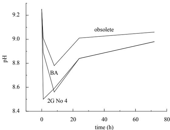
**Fig. 5.** pH versus time for Rouasan with different finishes SS 304 AISI
