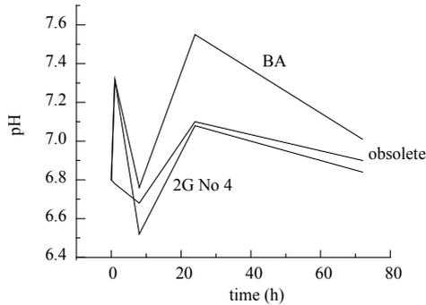
**Fig. 3.** pH versus time for Anasept with different finishes SS 304 AISI
