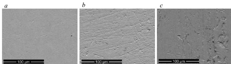
**Fig. 7.** SEM images on SS 304 AISI in Neoseptal: BA (a); obsolete (b); 2G No 4 (c)
