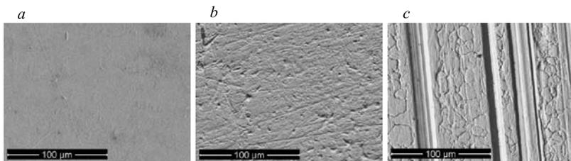
**Fig. 11.** SEM images on SS 304 AISI in Rouasan: BA (a); obsolete (b); 2G No 4 (c)
