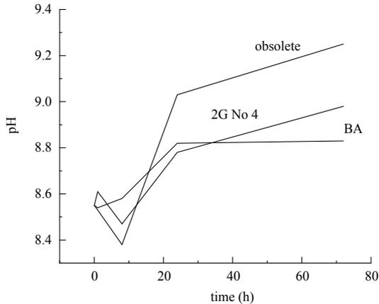
**Fig. 4.** pH versus time for Propano with different finishes SS 304 AISI
