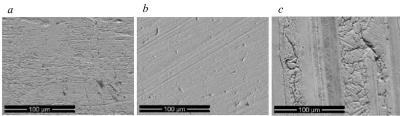
**Fig. 8.** SEM images on SS 304 AISI in Actisept: BA (a); obsolete (b); 2G No 4 (c)
