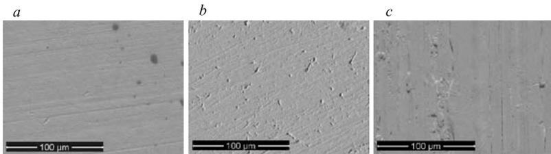
**Fig. 9.** SEM images on SS 304 AISI in Anasept: BA (a); obsolete (b); 2G No 4 (c)
