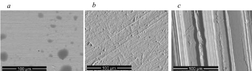
**Fig. 10.** SEM images on SS 304 AISI in Propano: BA (a); obsolete (b); 2G No 4 (c)
