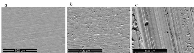
**Fig. 6.** SEM images on SS 304 AISI without disinfectants: BA (a); obsolete (b); 2G No 4 (c)
