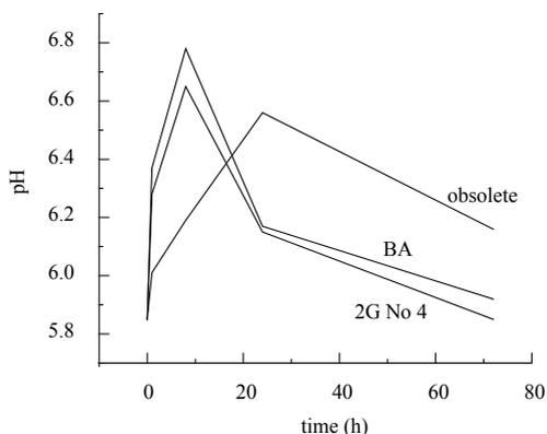
**Fig. 2.** pH versus time for Actisept with different finishes SS 304 AISI
