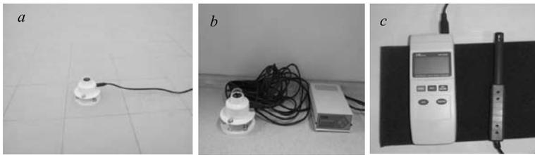
**Fig. 1.** Measurement equipments: 501 A UV biometers during measurements and experimental settings and a Lutron hygrometer
