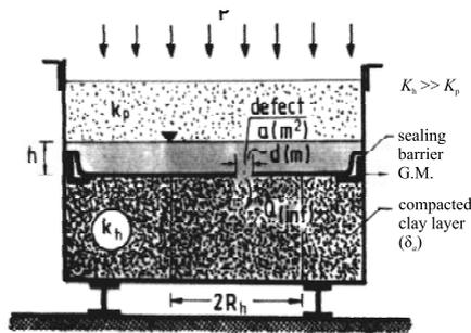
**Fig. 3.** Laboratory stand (source: A. Wehry et al., Ecotim 2000 Symposium, 2000, p.190)
