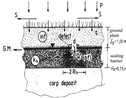
Fig. 2. The physical model (source: A. Wehry et al., Ecotim 2000 Symposium, 2000, p.189)
