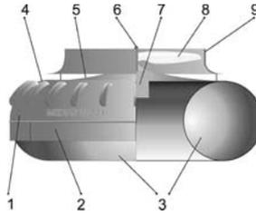
**Fig. 1.** Main components of the MEDIAS aerial vehicle (partially sectioned view)
