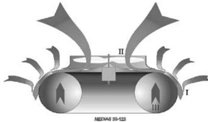
**Fig. 2.** Specific contribution of each device to the propulsion and sustentation of the MEDIAS aerial vehicle (the Coanda type)
