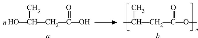
**Fig. 2.** Chemical structure of: 3-hydroxybutyrate-acid (a); poly(3-hydroxybutyrate) (PHB)<sup>3</sup> (b)
