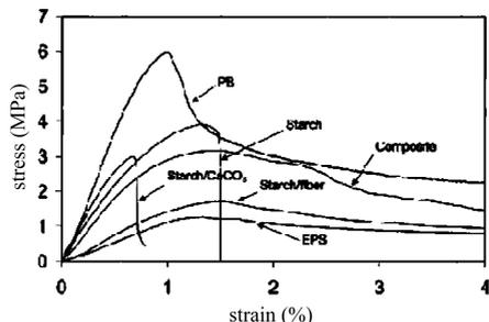
**Fig. 4.** Graph of flexural stress/strain curves for foam samples including extruded polystyrene (EPS), paperboard (PB) and baked foams made of formulations containing starch, starch and fibre (starch/fibre), starch and CaCO<sub>3</sub> (starch/CaCO<sub>3</sub>) or composites of starch, fibre and CaCO<sub>3</sub> (composite)<sup>16</sup>
