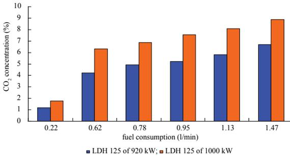
**Fig. 3.** CO<sub>2</sub> emissions of the 2 locomotives depending on fuel consumption
