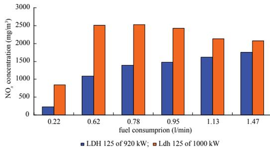
**Fig. 5.** NO<sub>x</sub> emissions of the 2 locomotives depending on fuel consumption
