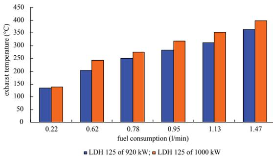
**Fig. 7.** Exhaust gas temperature depending on the fuel consumption
