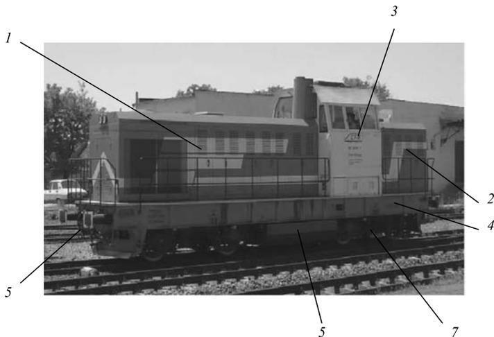
**Fig. 2.** Components of locomotive LDH 125 of 1000 kW (Ref. 4)
