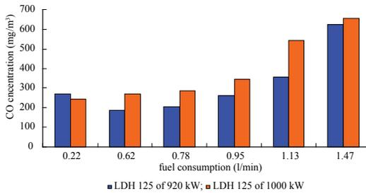
**Fig. 4.** CO concentration of the 2 locomotives depending on fuel consumption
