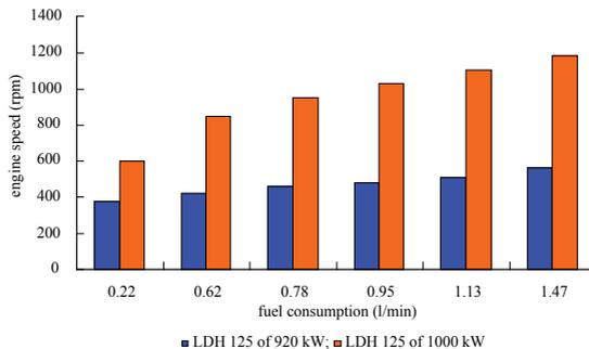
**Fig. 6.** Engine speed depending on fuel consumption
