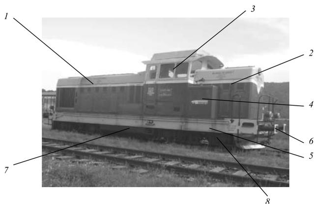
**Fig. 1.** Components of locomotive LDH 125 of 920 kW (Ref. 4)
