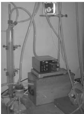
**Fig. 1.** Immobilised yeast bioreactor for continuous production of bio-ethanol
